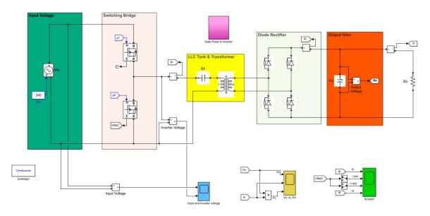
The input to the circuit is of 300V given by DC source. This is given to the inverter which converts DC to AC power. The inverter uses only two switches for the conversion. This becomes a reduced circuit. The pulses are  $180^{\circ}$  phase shifted. There two gate pulses given to it from the pulse generator of frequency 75 kHz as shown below.
