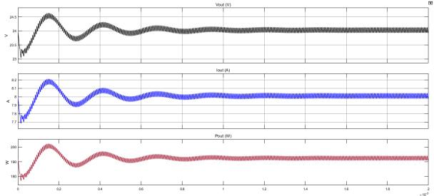
The first graph represented is an Output voltage of 24V, output current of 8A and the total output power of 192W.
